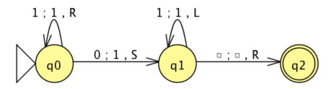
The TM starts in the initial state  $q_0$ , positioned on the leftmost of a string of 1's If it sees a 1, it writes a 1, moves right, and stays in state  $q_0$
